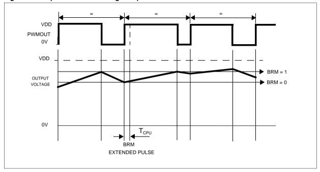
Figure 35. Graphical Representation of 4-Bit BRM Added Pulse Positions
