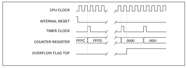
Figure 19. Counter Timing Diagram, internal clock divided by 8
