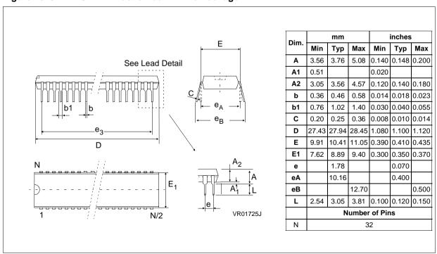
Figure 41. 32-Pin Shrink Ceramic Dual In-Line Package
