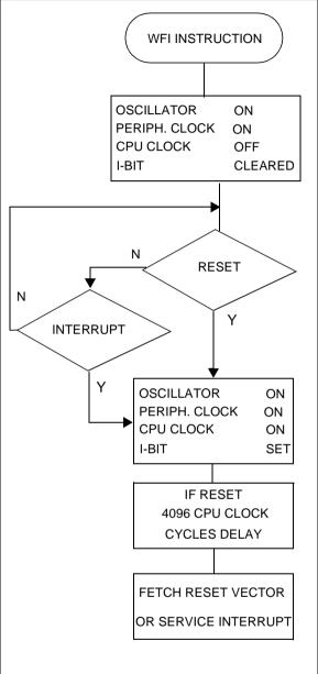
**Note:** Before servicing an interrupt, the CC register is pushed on the stack. The I-Bit is set during the interrupt routine and cleared when the CC register is popped.
