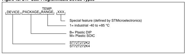
**Note:** The ST72E272K4D0 (32-pin ceramic SDIP) is used as the EPROM version for the above devices. The EPROM devices are tested for operation at 25 °C only.
