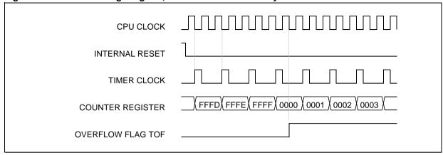
Figure 18. Counter Timing Diagram, internal clock divided by 4
