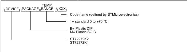
Figure 43. OTP User Programmable Device Types
