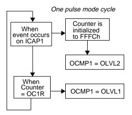
Then, on a valid event on the ICAP1 pin, the counter is initialized to FFFCh and OLVL2 bit is loaded on the OCMP1 pin. When the value of the counter is equal to the value of the contents of the OC1R register, the OLVL1 bit is output on the OCMP1 pin, (See Figure 24).
