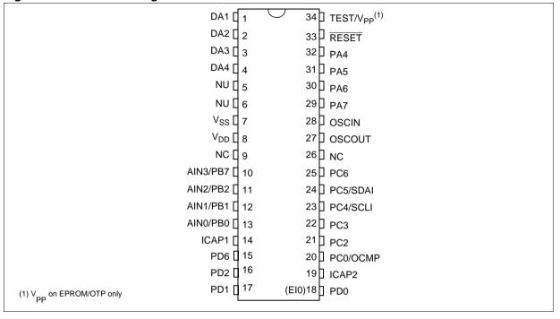
Figure 3. 32-Pin SDIP Package Pinout
